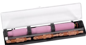
AK3C For A-200 Series, A-250 Series and W-350 Series. Includes one short back cap, one of each size (#5, #6, #8) alumina nozzle, and one of each size (1/16, 3/32, 1/8 inch) of the following: collet, collet body, and 7-inch 2% ceriated tungsten electrode.
