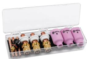
AK3GL For A-150, A-200 and A-250. Includes one short back cap, one of each size (#6, #7, #8) alumina nozzle, and one of each size (1/16, 3/32, 1/8 inch) of the following: gas lens, collet, and 7-inch 2% ceriated tungsten electrode.
