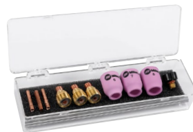
AK4GL For W-200, W-225, W-250, W-280 and W-375. Includes one short back cap, one of each size (#6, #7, #8) alumina nozzle, and one of each size (1/16, 3/32, 1/8 inch) of the following: gas lens, collet, and 7-inch 2% ceriated tungsten electrode.
