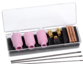
AK18C For W-400 Super Cool. Includes one short back cap, one of each size (#6, #7, #8) alumina nozzle, one of each size (3/32, 1/8 HD, 5/32 HD) collet, one of each size (.020-1/8 inch, 1/8-3/16 inch) collet body, and one of each size (3/32, 1/8, 5/32 inch) 7-inch 2% ceriated tungsten electrode.
