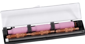
AK2C For A-150 Series. Includes one short back cap, one of each size (#4, #5, #6) alumina nozzle, and one of each size (.040, 1/16, 3/32 inch) of the following: collet, collet body, and 7-inch 2% ceriated tungsten electrode.
